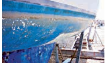
Paint blisters and lifts
