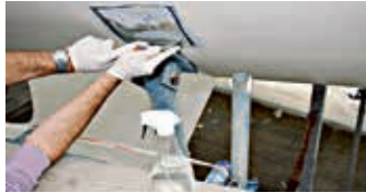
Wet scrape to remove old antifouling
